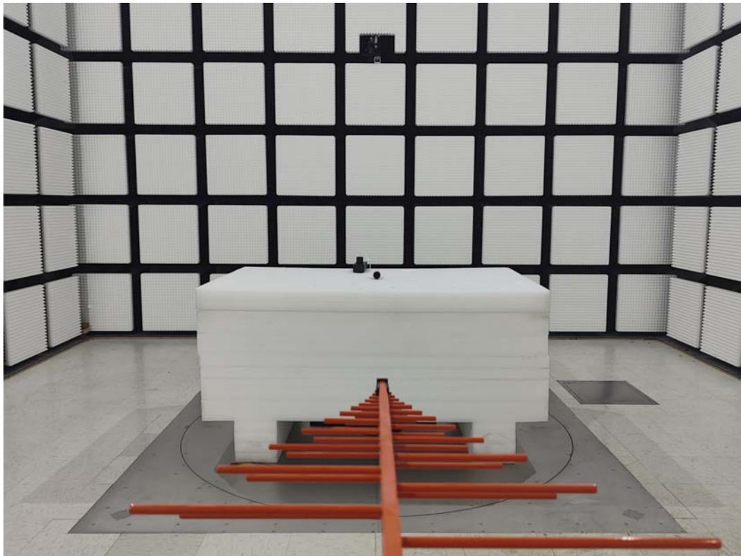
Radiated Emission Above 1GHz View
