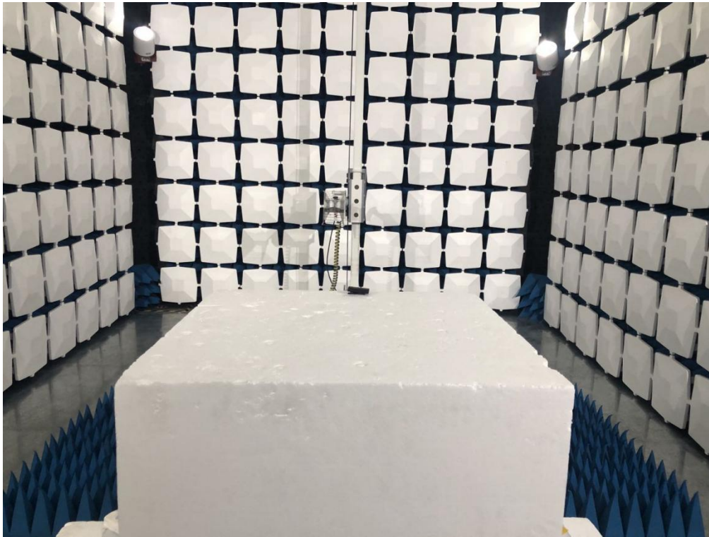
Above 1GHz for radiated emission test setup
