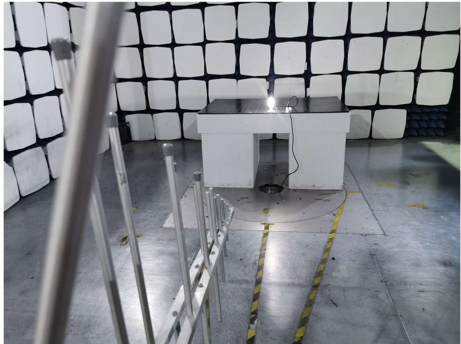
Radiation Emission Test Setup (30MHz to 1GHz)
