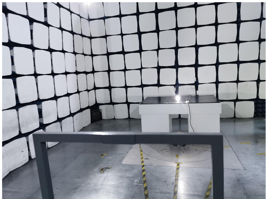
Radiation Emission Test Setup (Below 30MHz)
