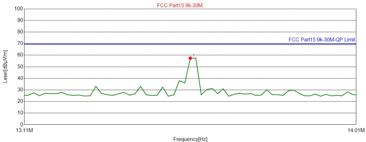
Margin [dB] =Limit [dB $\mu$ V/m] – Level [dB $\mu$ V/m]
