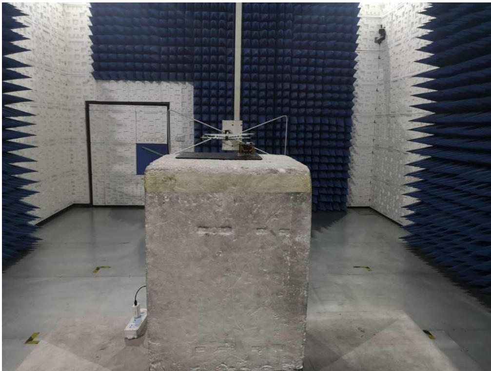
FCC RADIATED EMISSION TEST SETUP 30MHz-1GHZ
