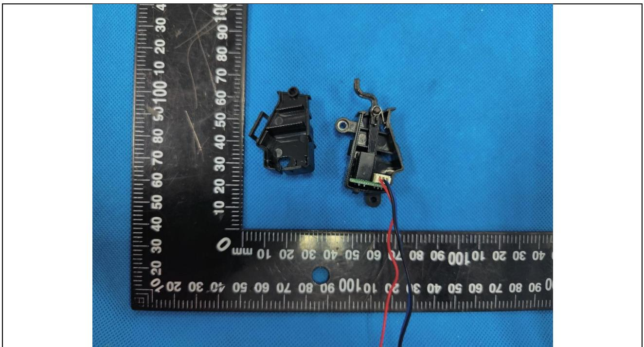
Details of: PCB view for Sensitive switch
