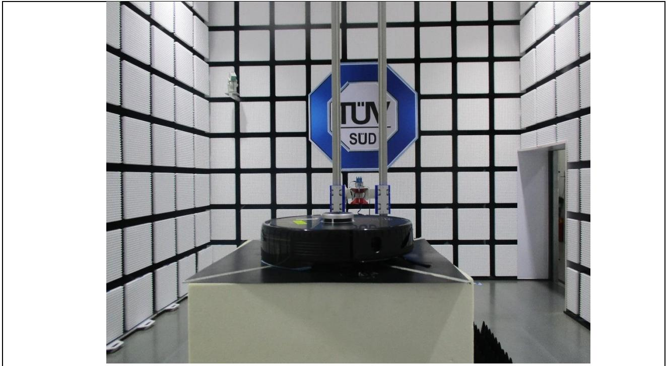
Test setup of: Spurious Radiated Emissions (Above 18 GHz)
