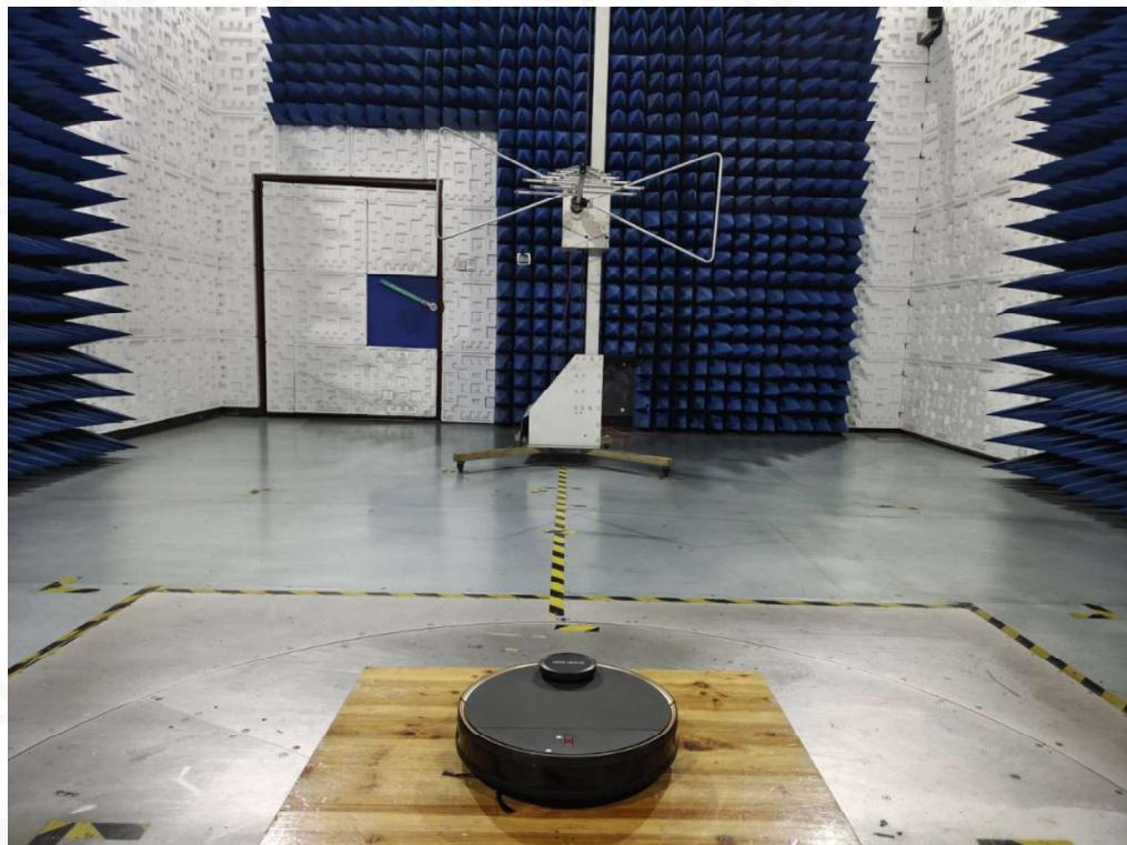
**FCC RADIATED EMISSION TEST SETUP ABOVE 1GHZ**
