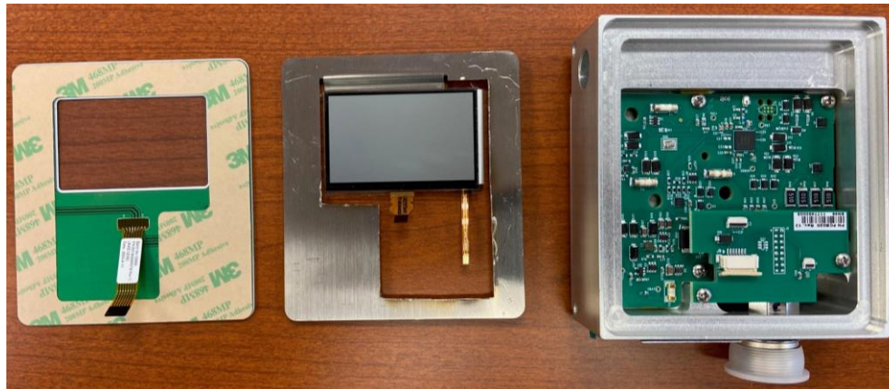
Circuit Boards as installed (Plate and Cover unstalled for photo)
