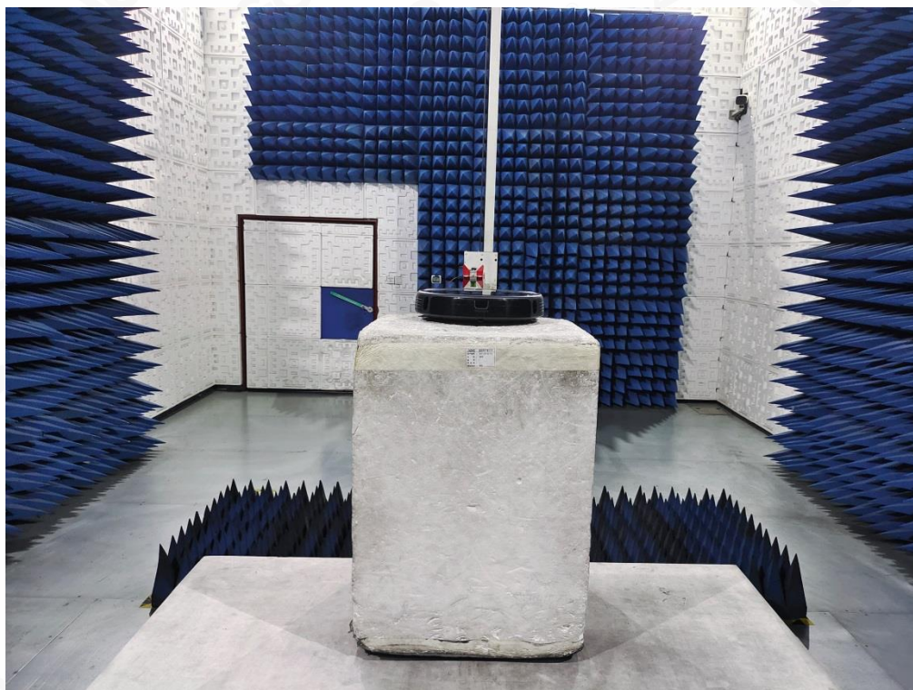
FCC RADIATED EMISSION TEST SETUP ABOVE 1GHZ
