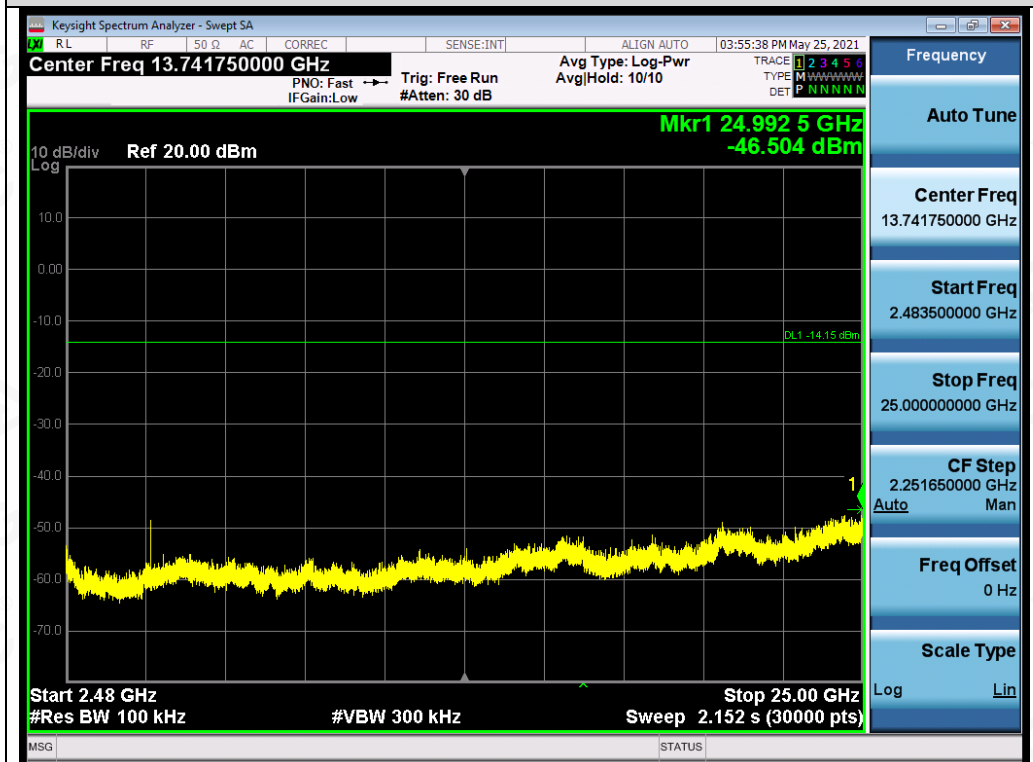
Test_Graph_802.11b_ANT1_2437_1Mbps_Higher Band Emissions
