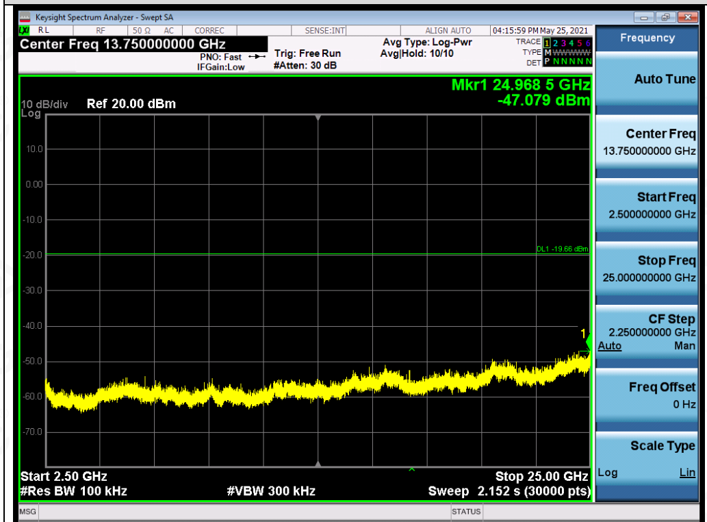
Test_Graph_802.11n20_ANT1_2462_MCS0_Higher Band Emissions
