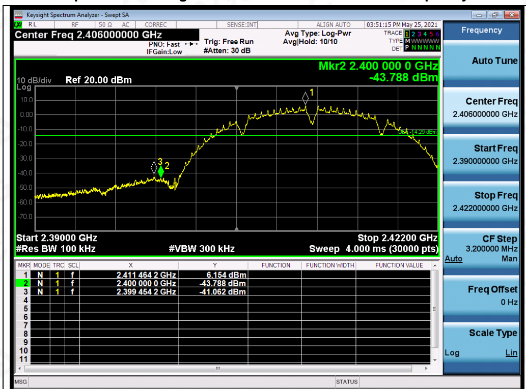
Test_Graph_802.11b_ANT1_2412_1Mbps_Lower Band Edge Emissions
