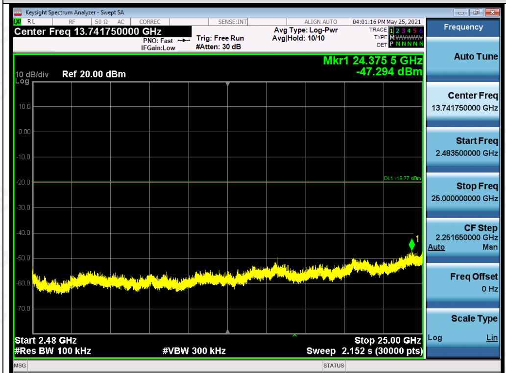
Test_Graph_802.11g_ANT1_2412_6Mbps_Higher Band Emissions
