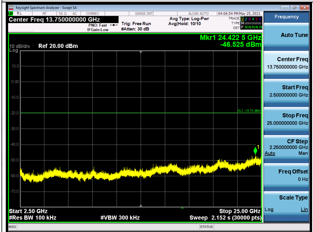
Test_Graph_802.11g_ANT1_2462_6Mbps_Higher Band Emissions
