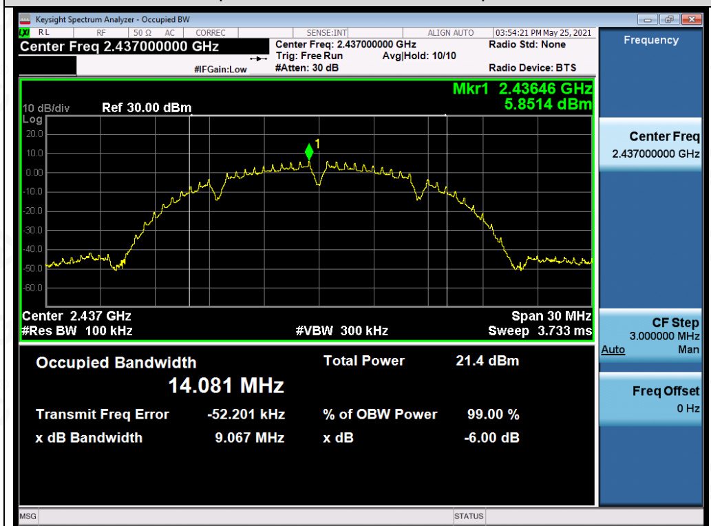
Test_Graph_802.11b_ANT1_2437_1Mbps_DTSBW
