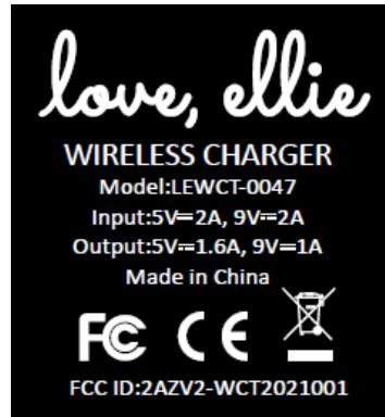
Specifications: Text is Black in color and justified. Labels are printed in indelible ink on permanent adhesive silk-screened onto the EUT or shall be affixed at a conspicuous location on the EUT.
