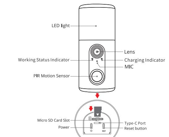
**CAUTION:** Please insert the Micro SD Card according to the direction shown in the diagram. Micro SD Card might JAM if inserted incorrectly and device could be damaged.
