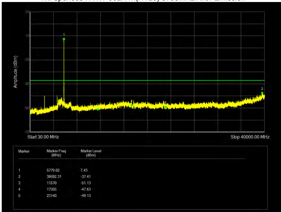
Tx. Spurious NVNT 802.11n(HT20) 5785MHz Ant1 Emission
