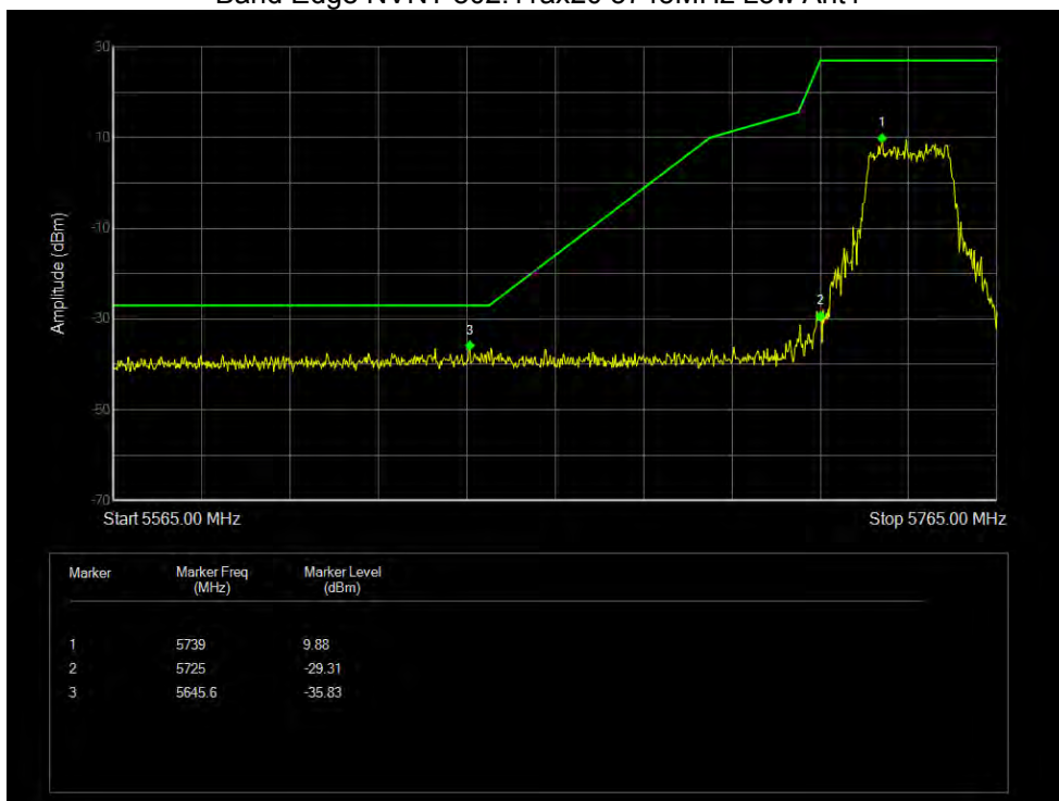
Band Edge NVNT 802.11ax20 5825MHz High Ant1
