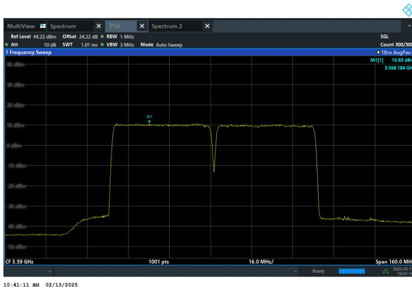
**SAS Granted MaxEIRP 35 [dBm/MHz]****UUT Center Frequency 3590 MHz, Bandwidth 80 MHz, MaxEIRP 34.39 [dBm/MHz]****TX 0**
