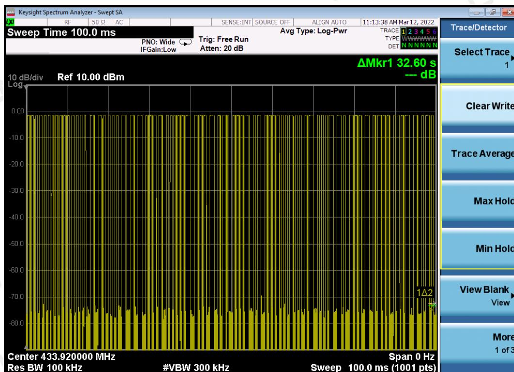
The graph shows the duration of 'on' signal. From marker 1 to marker 2, duration is 1.08ms.
