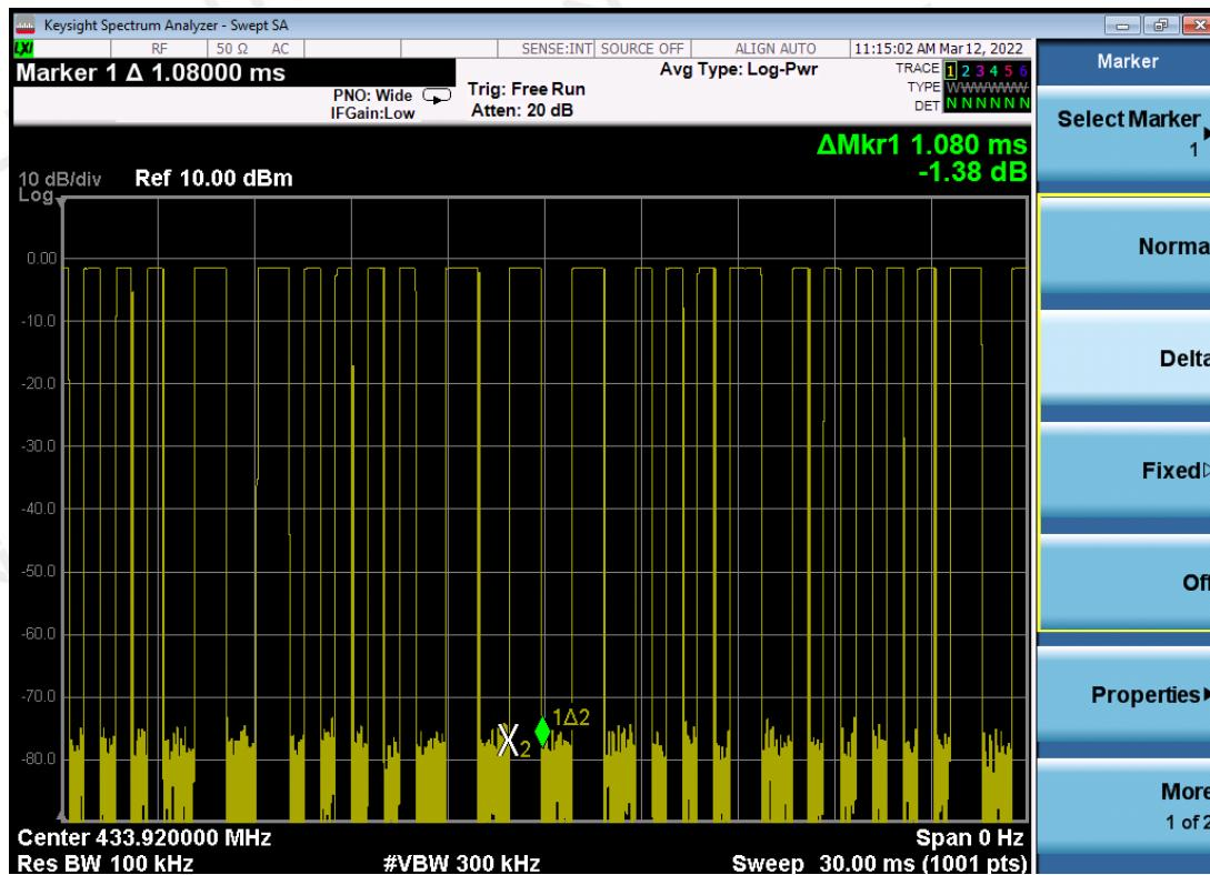
The graph shows the duration of 'on' signal. From marker 1 to marker 2, duration is 600μs(0.6ms).
