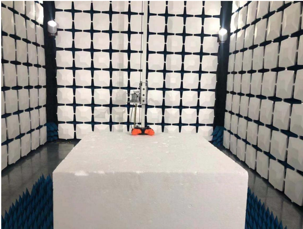
Above 1GHz for radiated emission test setup
