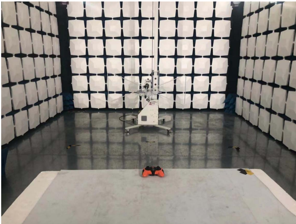
Below 1GHz for radiated emission test setup
