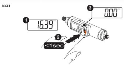
This function is recommended when the zero point is frequently repositioned (for example: comparative measurements)
