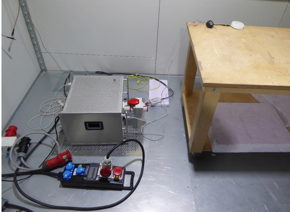
AC Mains conducted emissions setup for EUT2 with PA2
