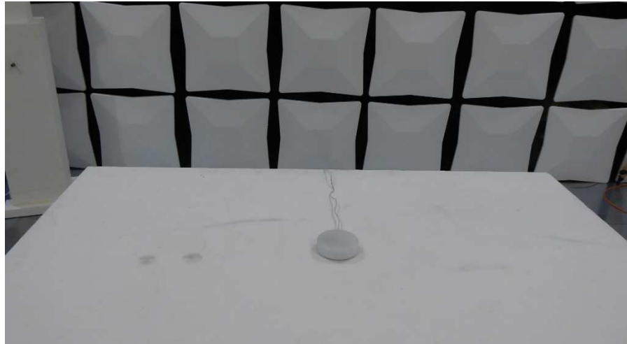
Setup for measurements below 1 GHz
