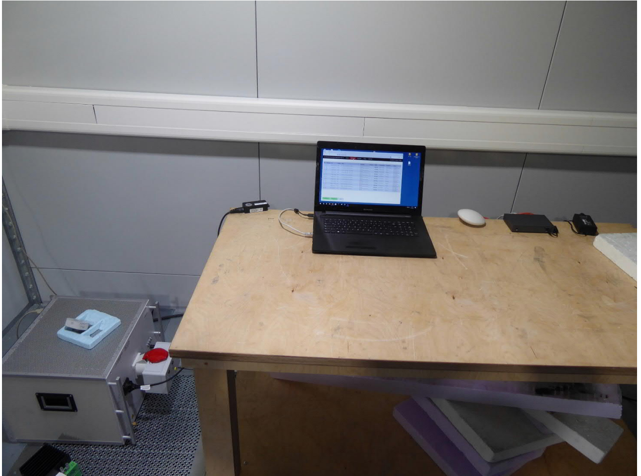
AC Mains conducted emissions setup for EUT with connector board 2
