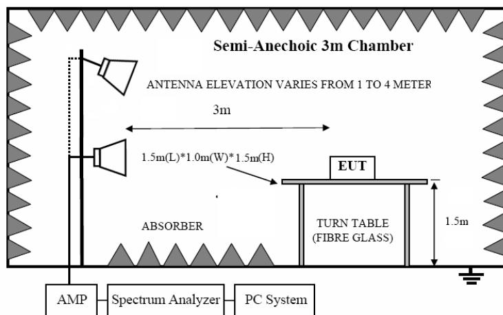
Note: For harmonic emissions test a appropriate high pass filter was inserted in the input port of AMP.
