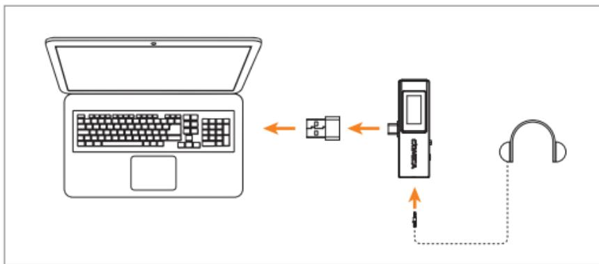
.Connect the receiver and USB-A device via the USB C-USB A adapter
