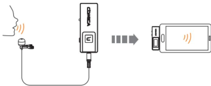
The transmitter audio is transmitted to the receiver unidirectionally, audio can only be monitored in receiver
