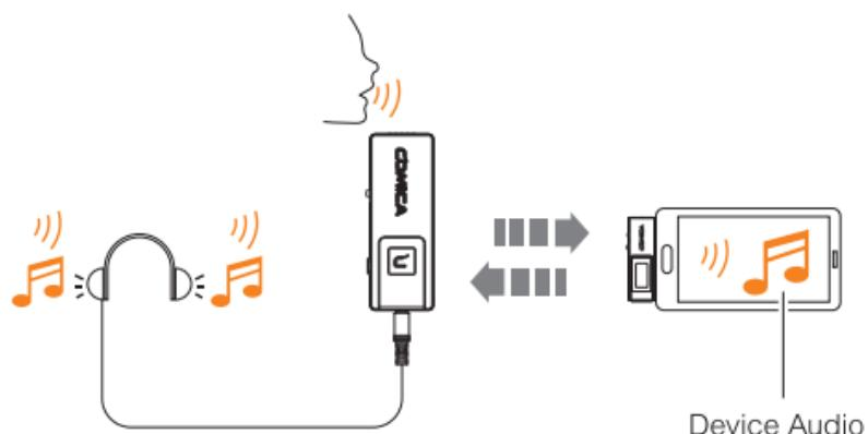
Two way transmission of audio between transmitter and receiver, audio can be monitored in transmitter and receiver
