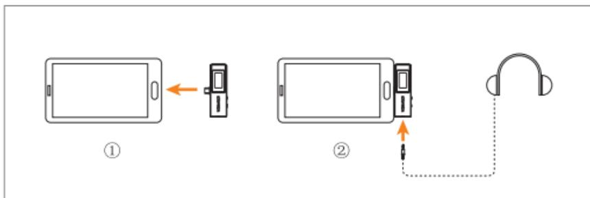
.Insert the receiver to the USB-C device
