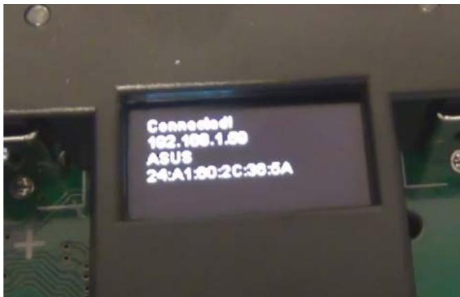
The connected message and the IP address should appear on the display in a few seconds after the WPS has been activated on your router, and the MegaCell Charger completed the connection.
