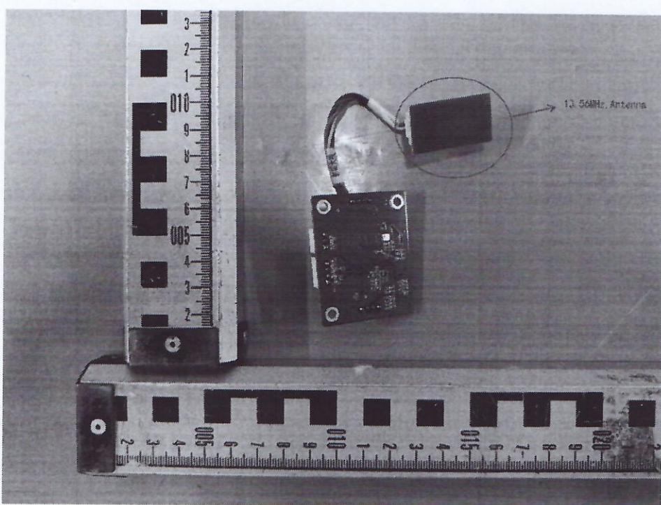
Antenna transmission frequency: 13.56MHz
