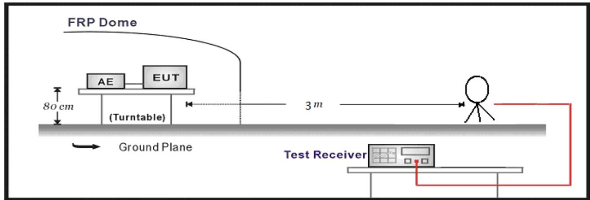
Below 1GHz Test Setup:
