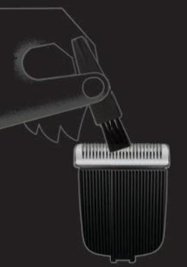
1 Remove blade. Using the cleaning brush, brush hair trimmings out of blade slots and in between blade teeth.
