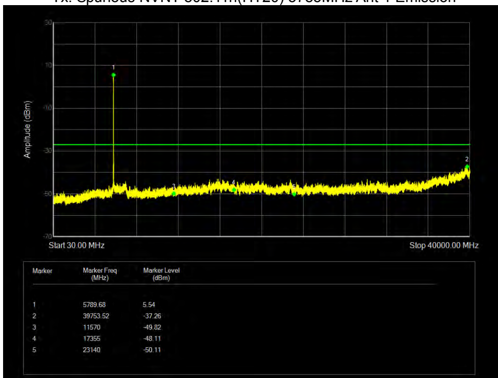
Tx. Spurious NVNT 802.11n(HT20) 5825MHz Ant 1 Emission
