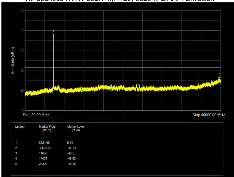
Tx. Spurious NVNT 802.11n(HT20) 5825MHz Ant 1 Emission
