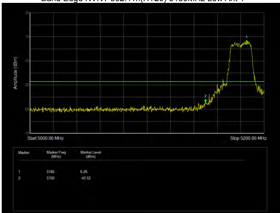
Band Edge NVNT 802.11n(HT20) 5180MHz Low Ant 1
