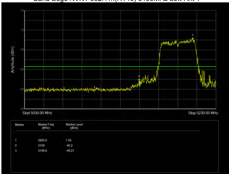
Band Edge NVNT 802.11n(HT40) 5190MHz Low Ant 1
