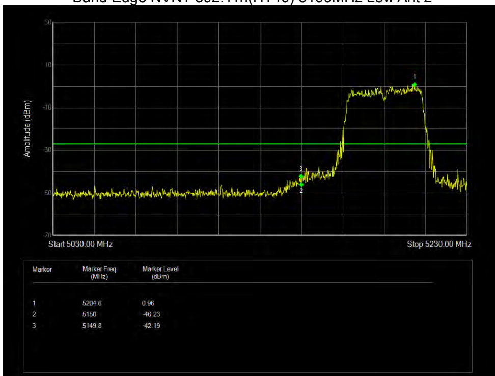
Band Edge NVNT 802.11n(HT40) 5190MHz Low Ant 2
