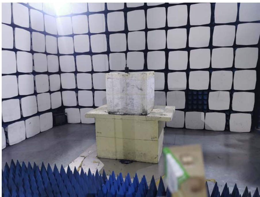
Radiation Emission Test Setup (Above 18GHz)
