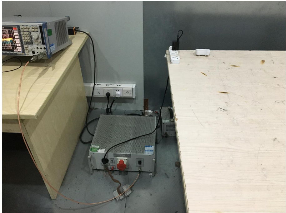
Conducted Emission Test Setup
