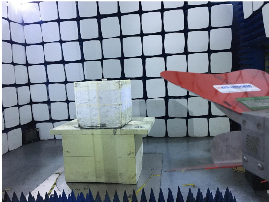
Radiation Emission Test Setup (1GHz to 18GHz)
