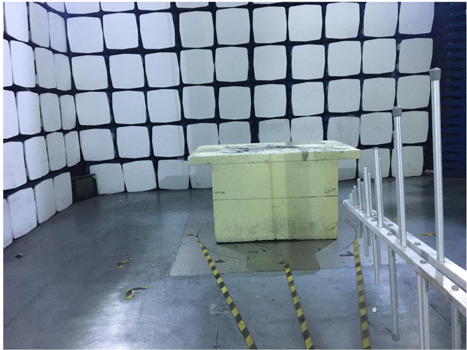
Radiation Emission Test Setup (30MHz to 1GHz)
