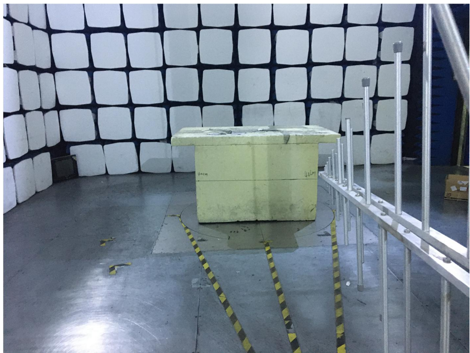
Radiation Emission Test Setup (30MHz to 1GHz)
