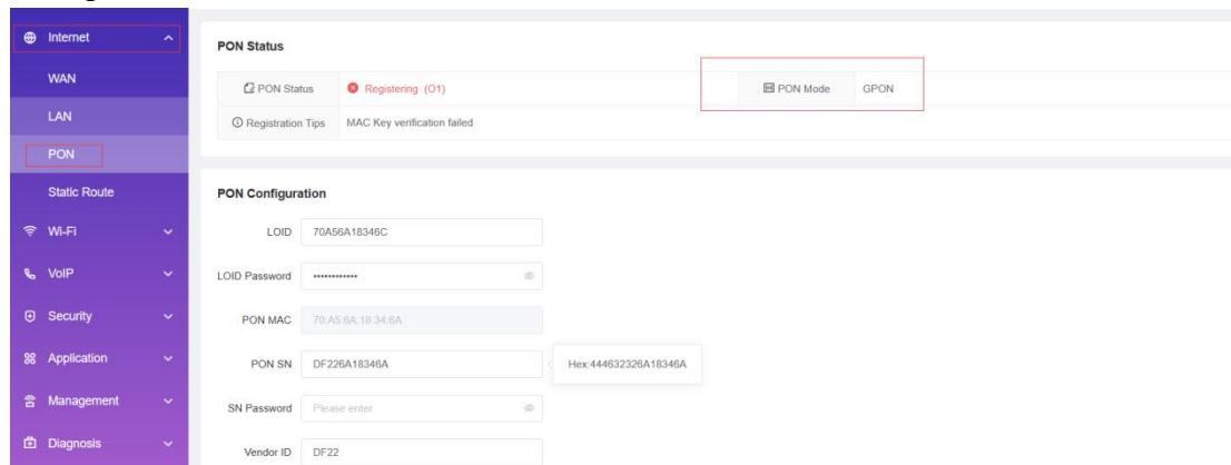
The screenshot shows the ONU PON status configuration interface. The left sidebar has a 'PON' tab selected. The main area has two sections: 'PON Status' and 'PON Configuration'. In 'PON Status', the 'PON Mode' is set to 'GPON' and the status is 'Registering (O1)'. In 'PON Configuration', fields include LOID (70A56A18346C), LOID Password (redacted), PON MAC (70:A5:6A:18:34:6A), PON SN (DF226A18346A), SN Password (redacted), and Vendor ID (DF22).
