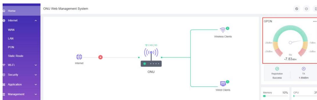
The screenshot shows the ONU Web Management System interface. The left sidebar has a 'PON' tab selected. The main area displays a network diagram with an 'Internet' connection to an 'ONU' device, which then connects to 'Wireless Clients' and 'Wired Clients'. To the right is a circular 'GPON' power meter showing Rx power at -7.83dBm and Tx power at 1.89dBm. Below the meter, status indicators show 'Registration Success' and resource usage for 'Memory' (10%) and 'CPU' (3%).
