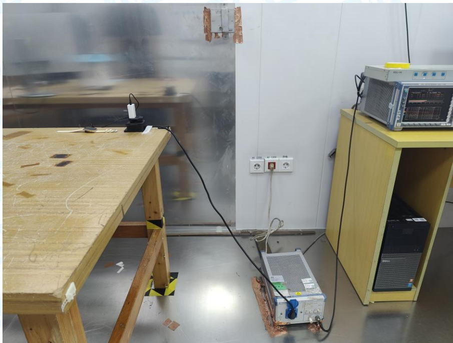
Photo of Setup for Conducted Emission
