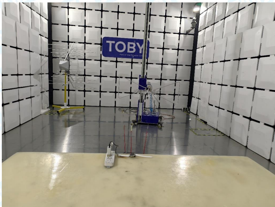
Radiated Emission Test Setup-Below 1G
