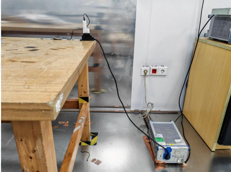
Photo of Setup for Radiated Emission (30MHz~1GHz)
