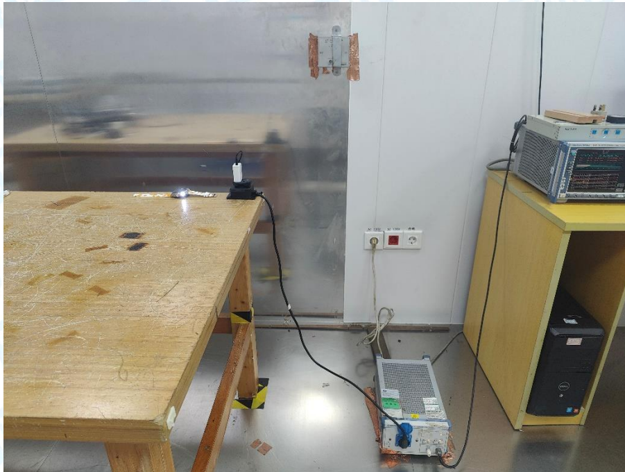
Photo of Setup for Radiated Emission (30MHz~1GHz)
