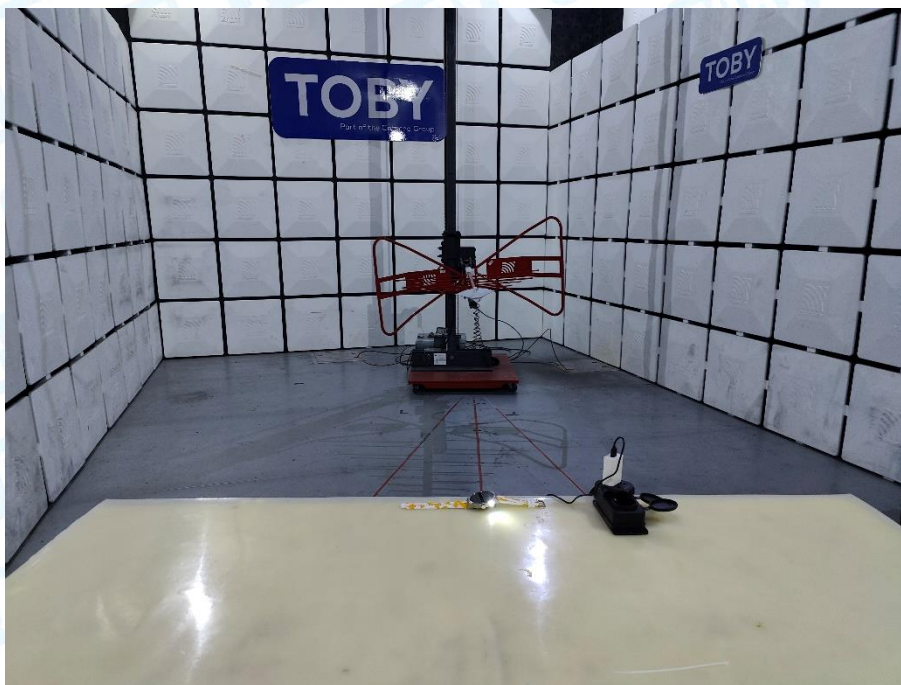
Photo of Setup for Radiated Emission (30MHz~1GHz)
