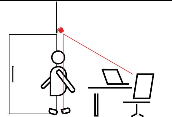
Traffic Mode provides aggregated totals of 'in' and 'out' movements based on a sensor's orientation, a user-defined door line, and the direction of entry. It is recommended to mount the sensor above entrances using either a Wall Mount or Ceiling Mount for optimal performance.
