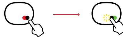
When switched on, unpaired Heatic Sensors set to the default Network ID will flash a yellow LED. If this does not occur, first ensure that the batteries are correctly installed. For further assistance, contact your Butlr representative or submit a support ticket.
