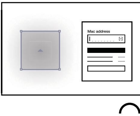
Update the virtual placeholder to accurately reflect device-specific information, such as the MAC address, serial number, installation height, orientation, mounting method, and precise location. Modify the device's custom fields as necessary.
