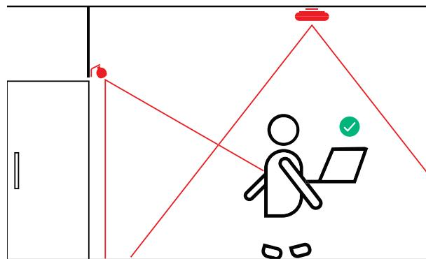
Use Studio and the materials provided by Butlr to verify the correct installation of devices and ensure data quality, optimizing sensor performance.
