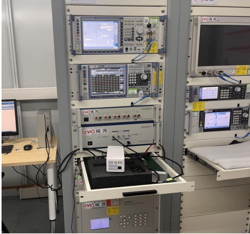
Radiated Test Setup(frequency range:30MHz-1GHz)
