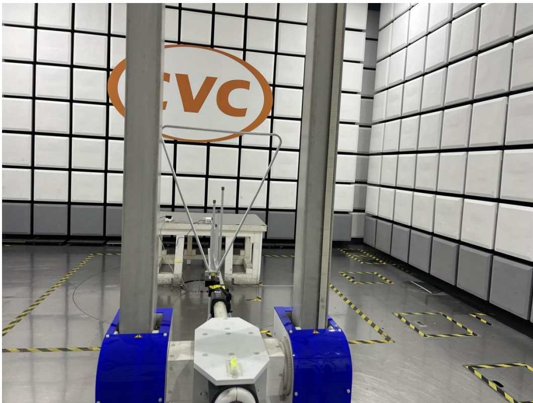
Radiated Test Setup(frequency range:30MHz-1GHz)
