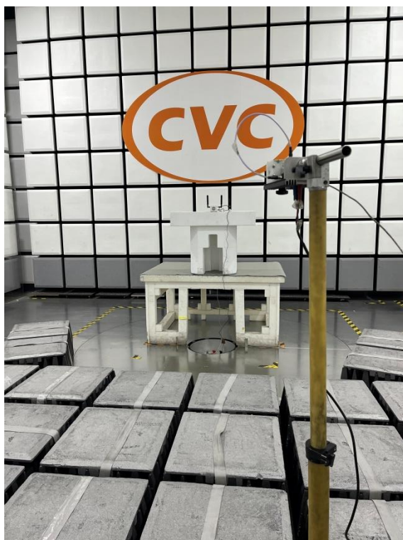
Radiated Test Setup(frequency range:18GHz-40GHz)
