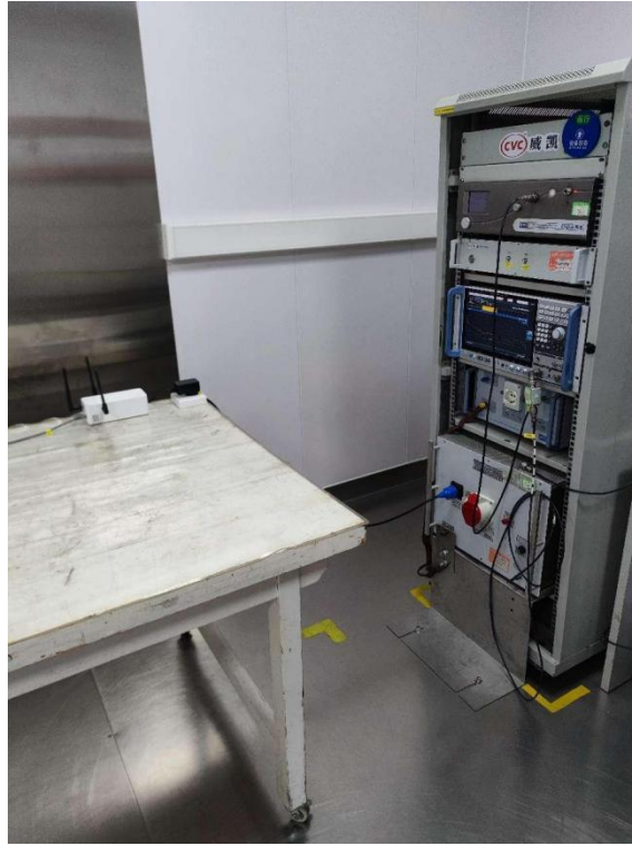
Conducted Emission Test Setup(30MHz to 26.5GHz)
