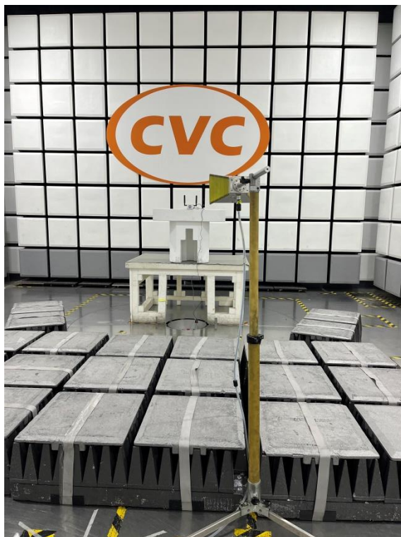
Radiated Test Setup(frequency range:18GHz-40GHz)
