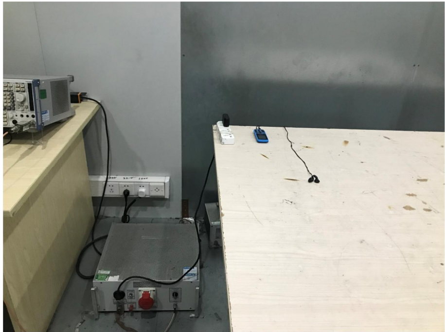
Conducted Emission Test Setup
