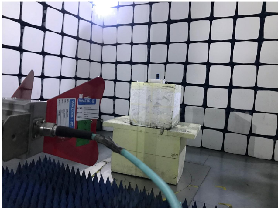
Radiation Emission Test Setup (1GHz to 18GHz)
