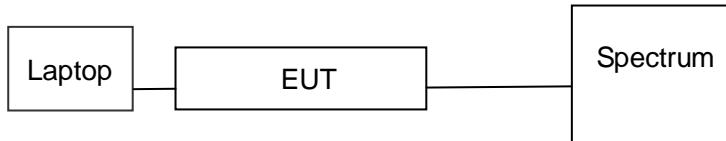
Note: 1. The EUT was used fully-charged battery programmed to be in continuously transmitting mode and the transmit duty cycle is not less than 98%.
