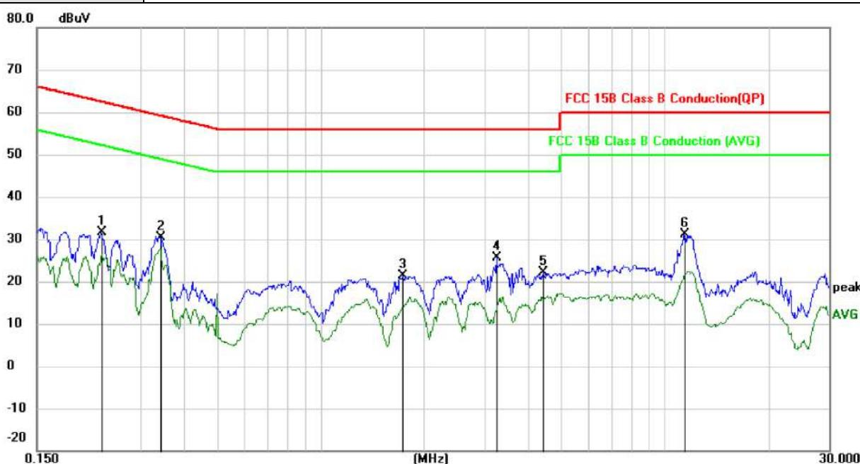
Remark: Factor = LISN factor + Cable Loss + Pulse limiter factor.
