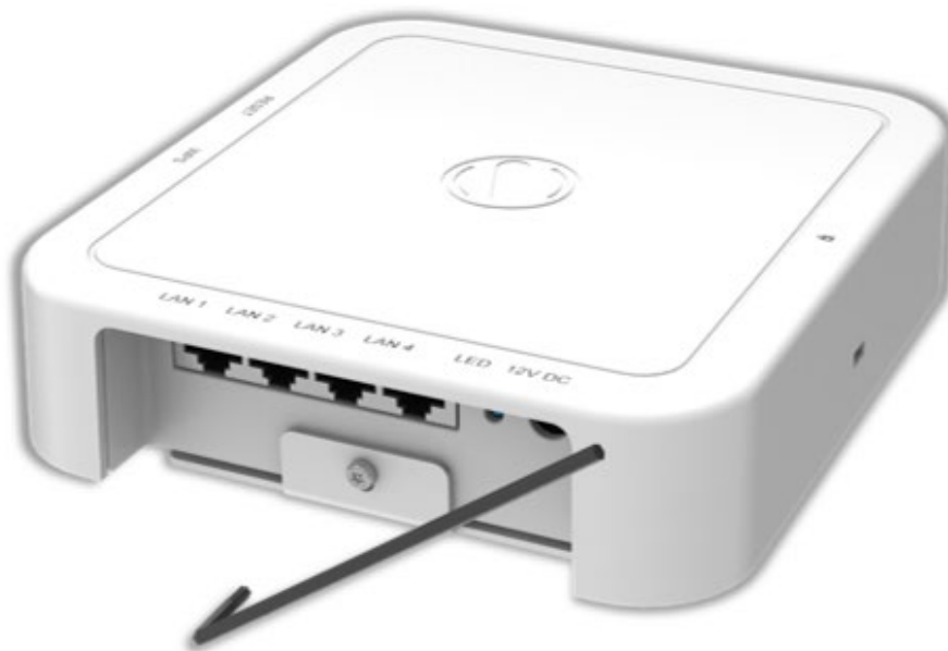
Figure 6: Unscrewing the Mounting Bracket of ion4xi_WP
