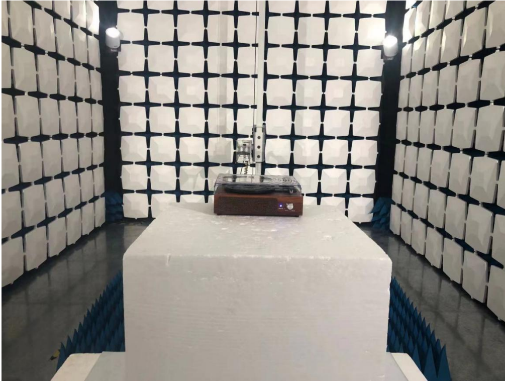
Above 1GHz for radiated emission test setup
