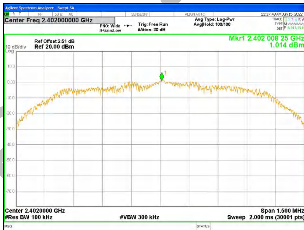
Tx. Spurious NVNT 2-DH1 2402MHz Ant1 Emission
