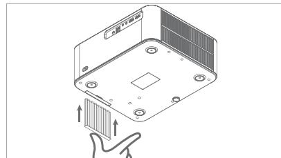
3. Reinstall the Dust Box: Once cleaned, place the dust box back into its original position.
