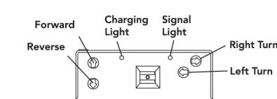
The RC Car moves forward and the headlights light up when the Forward button is pressed. The RC Car moves backward and the tail lights light up when the Reverse button is pressed.
