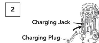
Insert the Charging Plug into the Charging Jack on the bottom of the RC Car. The Charging Light lights up to indicate that charging is in progress.
