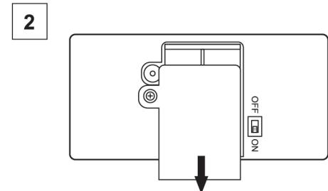
Use a Phillips screwdriver to remove the battery cover on the back of the remote control.
