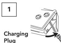
Open the Charging Plug cover as illustrated and remove the Charging Plug.
