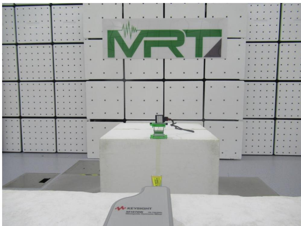
Description: Radiated Emission Test Setup for 110GHz ~ 140GHz
