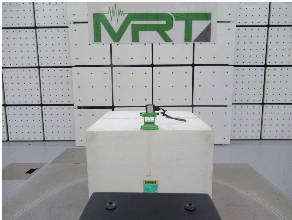
Description: Radiated Emission Test Setup for Above 140GHz
