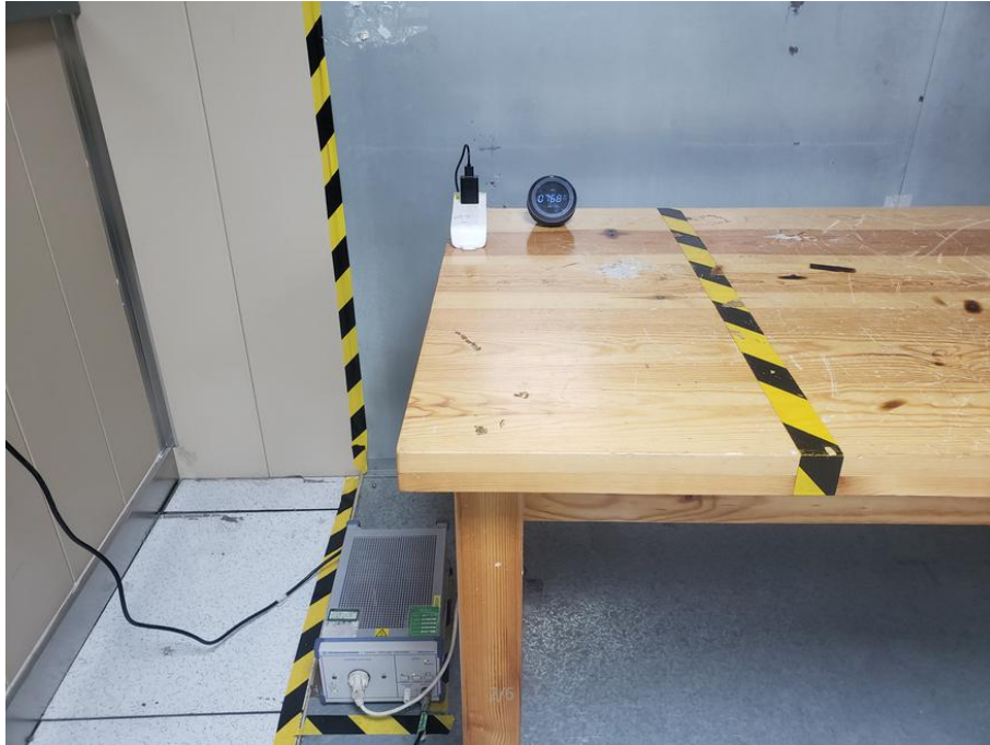
Radiated Emission below 1GHz
