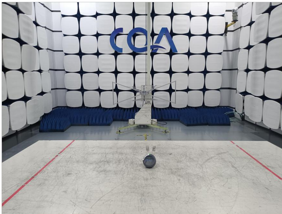
Radiated Emission below 1GHz
