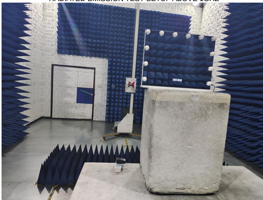
RADIATED EMISSION TEST SETUP ABOVE 1GHZ
