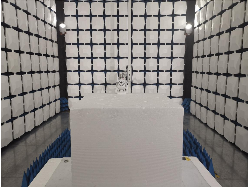
Above 1GHz for radiated emission test setup
